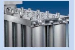
Detail of modular PSA aluminum banks based on single modules concept.
