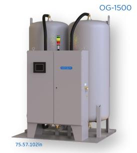
NOVAIR's oxygen generator series is the tried and true industry leader in standard O2 generating equipment. The OG extracts oxygen directly from the atmosphere and delivers it to any health or industrial application using Pressure Swing Adsorption (PSA) technology that can deliver a constant flow of up to 93% (+/-3%) oxygen purity at up to 55 PSI.
