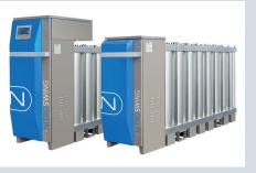
For large production capacities, a "Dual Bank" can be added consisting of a second PSA nitrogen generator without any PLC or power supply. The Master Dual Bank gets its power and control signals from the NITROSWING® PSA nitrogen generator through a single cable connection, with one master NITROSWING® PSA nitrogen generator controlling up to three Dual Banks simultaneously.
